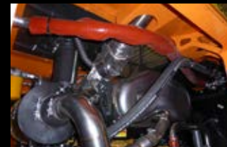
Second stage air filtration with ejector
