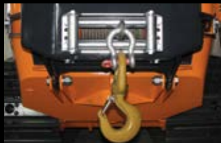
Rear winch with 6 t pulling power
